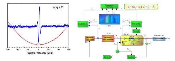
Figure 2 Left: Saturated absorption spectrum (red curve) and the respective 3f spectrum of the P(7) F1(1) component of the v3 band of CH4. The MIR frequency of the OPO is locked to the zero crossing of the 3f signal for absolute-frequency measurement of the absorption line center. Right: Experimental setup.
