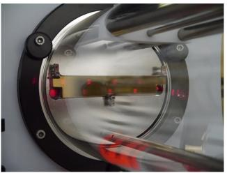
Figure 1: Spot pattern of reflections on the gold mirror of the White-cell within the path length calibration procedure by means of the laser distance meter approach.
